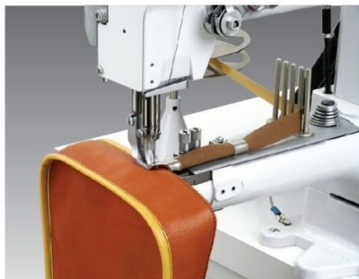
缝纫配件E5和滚边器用于面料的滚边 Sewing equipment E5 and moving binder for binding the fabric edges sewing equipment
